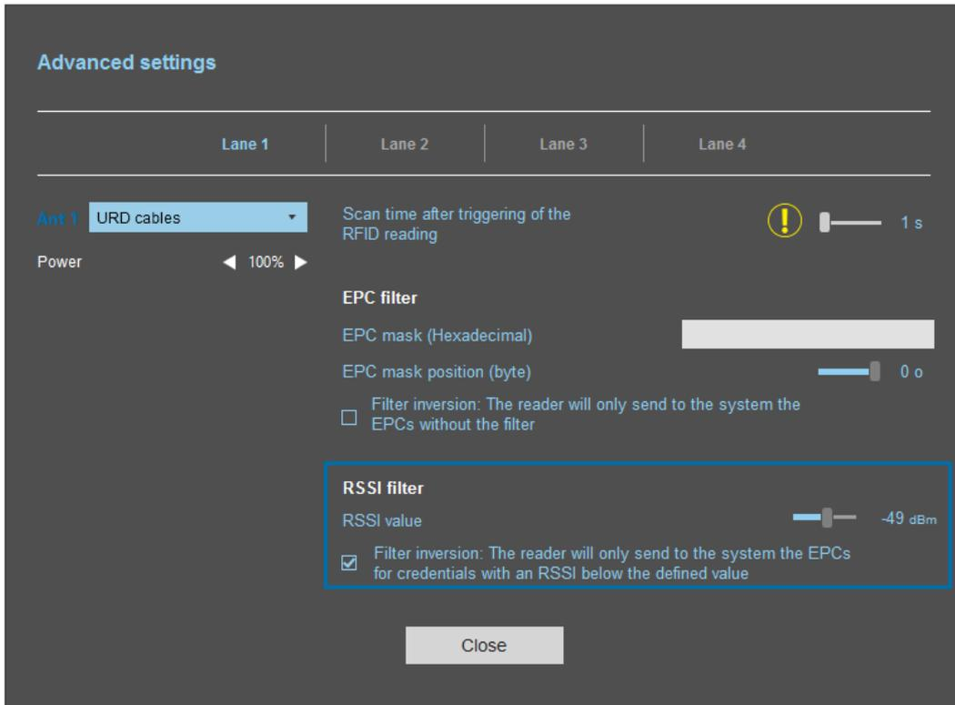
When “Inversion” is activated, tags with an RSSI lower than -49dBm are sent to the system. The others are not.
