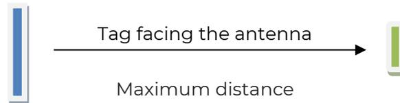
The distances in the technical specifications of readers are measured facing the reader, with the tag parallel to the antenna.
