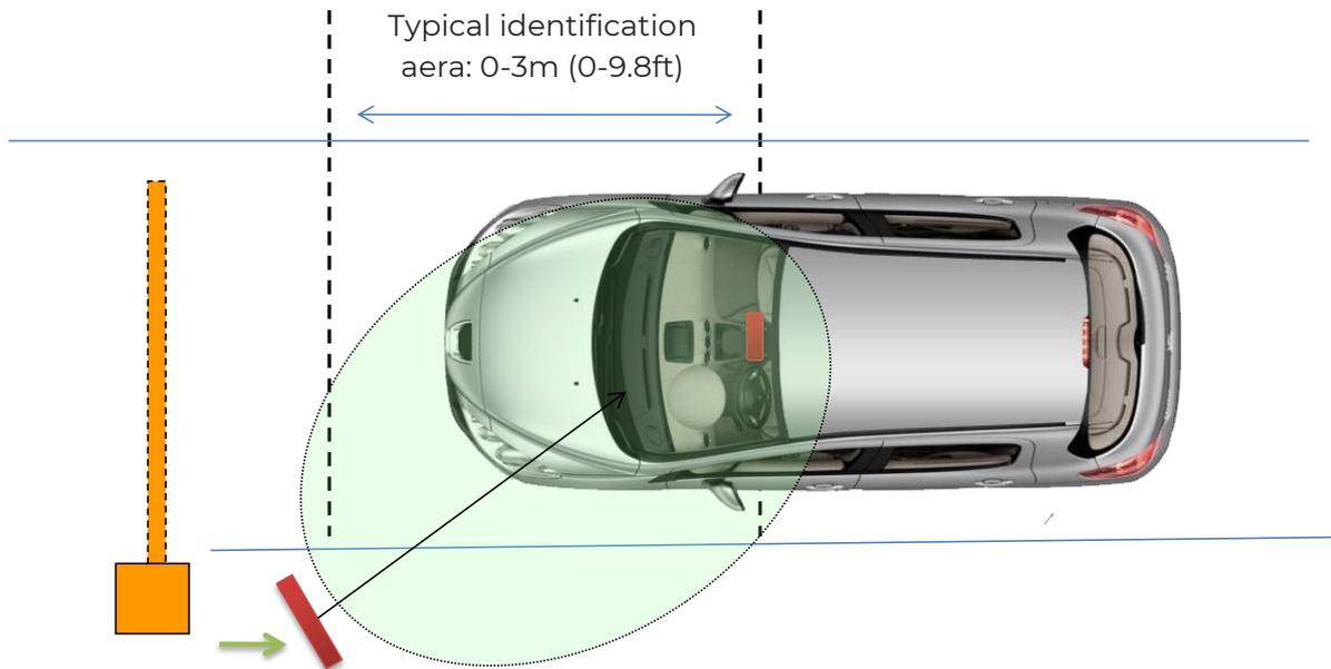
Installing the antenna at height allows it to be directed downwards in order to limit the reading distance on the ground and to avoid the unwanted detection of a second vehicle.
