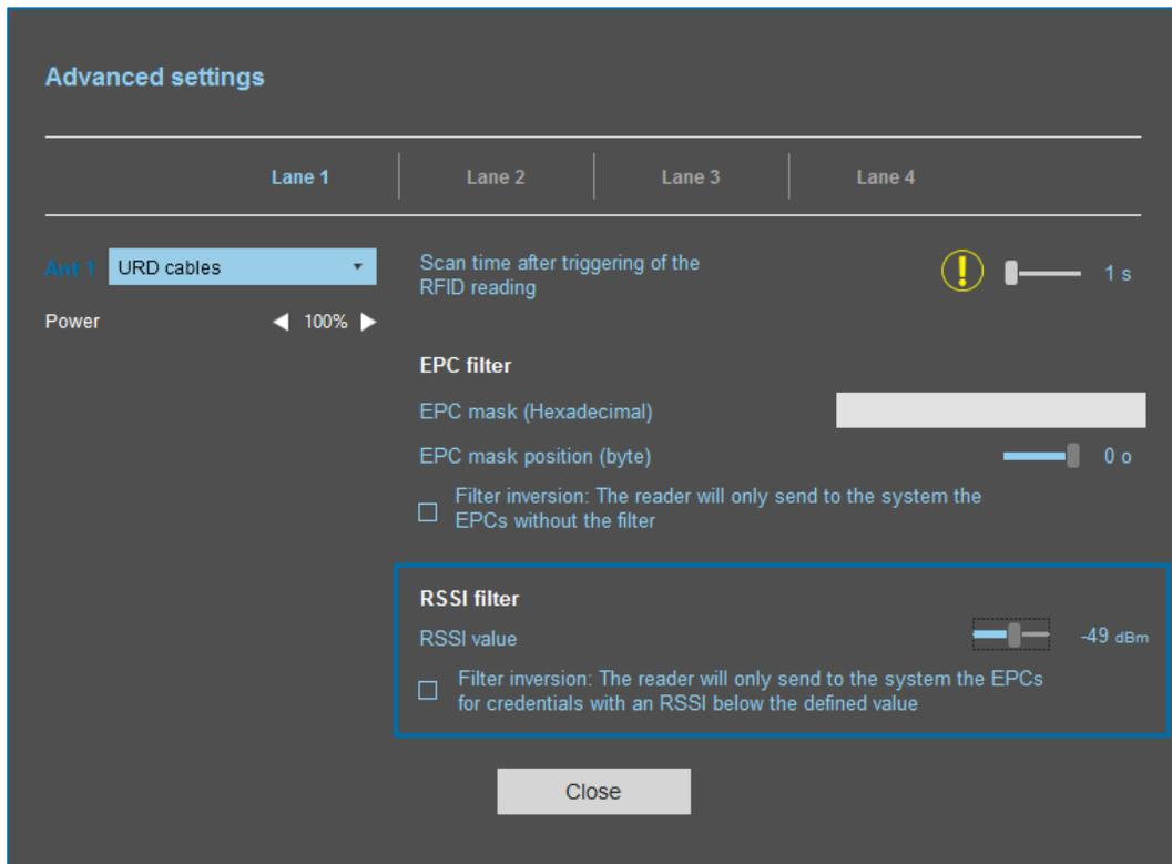
Tags with an RSSI higher than -49dBm are sent to the system. The others are not.
