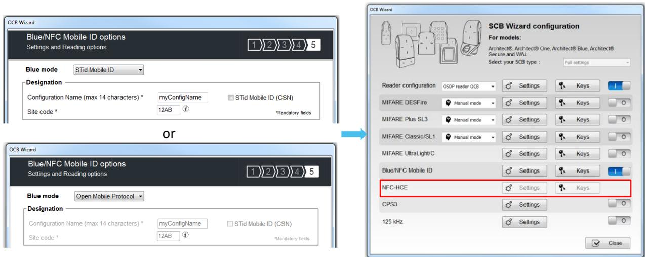
If “Orange Pack ID “ is activated it is possible to activate “NFC-HCE“, the parameters and keys are not greyed.
