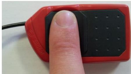
When the fingerprint is read, it is displayed on the window and the bar on the right shows the progress of the analysis.
